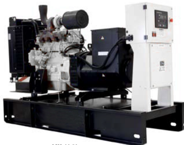
BCJD 90-50: engine 4045TF258, alternator UCI 224 G, control panel BC 7210
