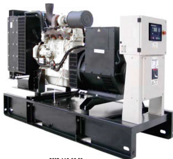
BCJD 110-50 E2: engine 4045 HFU 79, alternator UCI 274 C, control panel BC 7310
